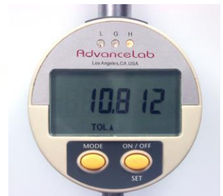
Gauge showing "H" for reading too High
