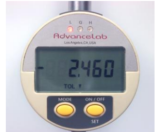
Gauge showing "L" for reading too Low
